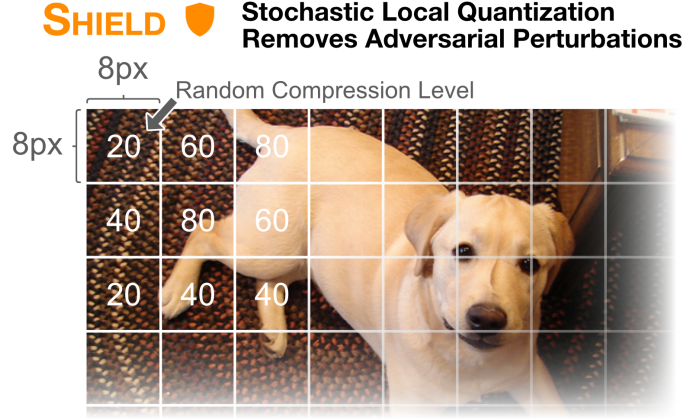
Figure 4.2: SHIELD uses Stochastic Local Quantization (SLQ) to remove adversarial perturbations from input images. SLQ divides an image into 8 \times 8 blocks and applies a randomly selected JPEG compression quality (20, 40, 60 or 80) to each block to mitigate the attack.
